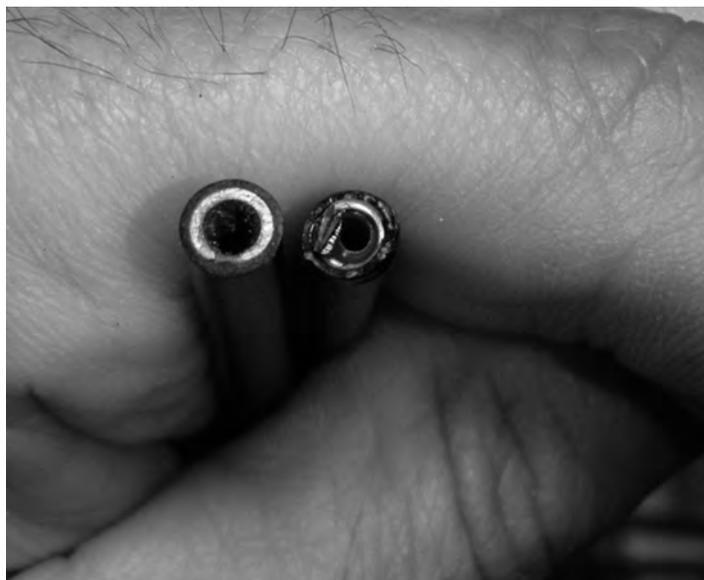
Make sure your cable housing is cut smoothly like the one on the left. The housing on the right has a burr that will cause poor shifting and abrade the cable.
