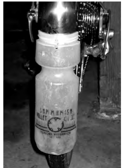
Top right: We give high marks to this RUSA motif submitted by Portland RBA Susan France. Middle: France's "Jingle Bells" flap, complete with tree ornaments. Bottom: Terry Zmrhal turned an old water bottle into a mudflap by cutting it in half.
