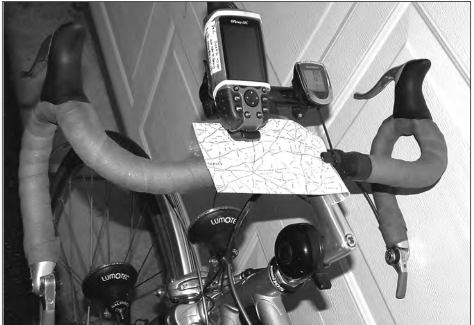
Note the bar-cons, map clip, GPS, space bar, dual Lumotec lights ...and a bell.
